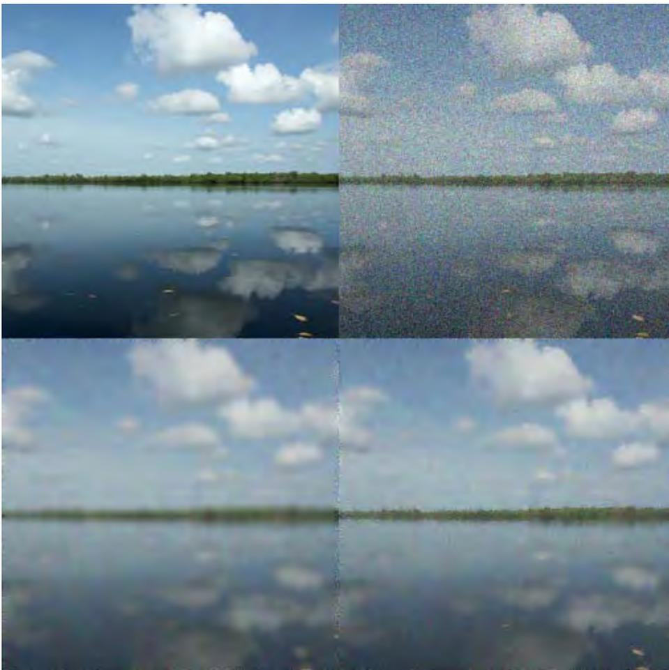
Abbildung 4-13: Original, Gaussian Noise, Arithmetic Mean Filter, MMSE Filter
