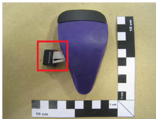
Figure 11.1: FCC picture - Vibratissimo Panty Buster. The debugging interface can be clearly seen
