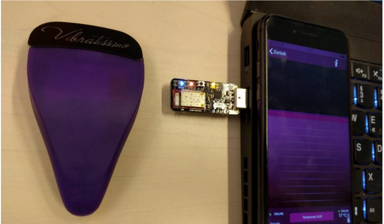
Figure 10.2: BluefruitLE Sniffer placed between the device to be attacked and the smartphone controlling the device to capture packets
