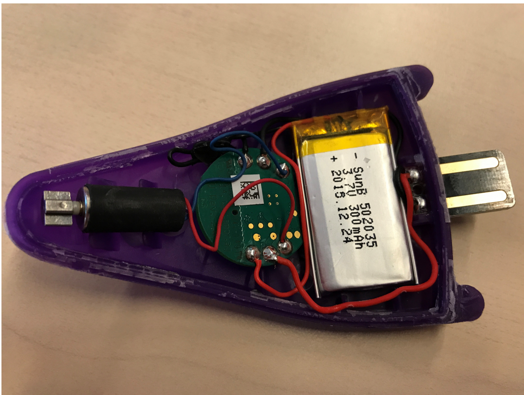
Figure 11.4: Disassembled panty buster with debugging interfaces
