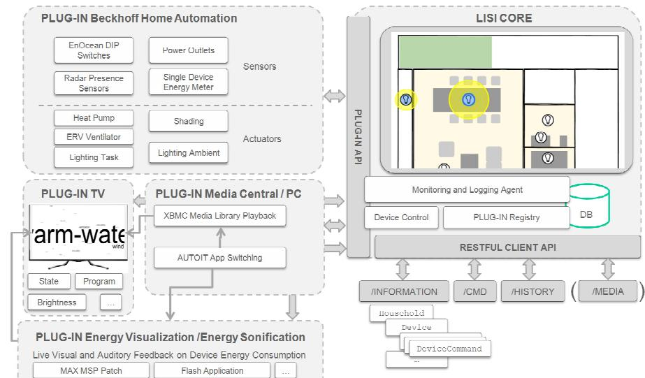
Figure 1 LISI Core – System architecture and various plug-ins (as used in the Solar Decathlon Team Austria's LISI smart home)
