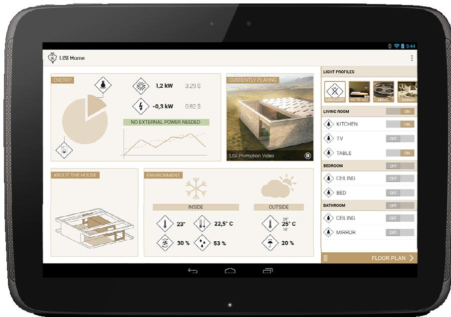
Figure 4 Control and Information Display that interacts with the LISI Core framework (done by Vienna University of Technology INSO-DECO, partner of the Solar Decathlon Team Austria)
