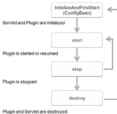
Figure 3 Plug-in lifecycle phases
