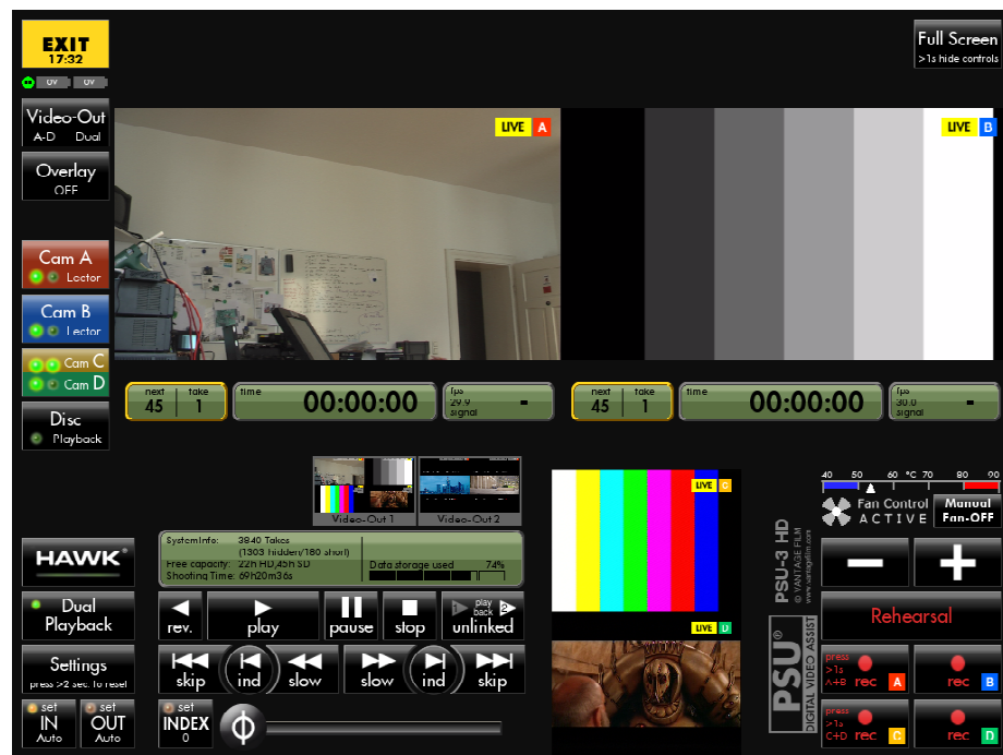
Figure 2 PSU®-3X HD main screen recording four cameras simultaneously
